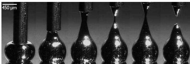
Figure 3.14: Image of the step by step formation of an EGaIn tip (Figure reprinted with permission from. [2] Copyright © 2007, John Wiley and Sons).
